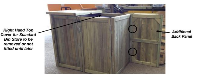
**Step 3:** Fix the Additional Side Panel to the Additional Back Panel using 3 no M5 x 90mm screws. Looking from the inside of the Additional Bin Store the Additional Side Panel has markings for the Tie Bars on the right hand corner. Make sure that markings are in the right place when positioning the Additional Side Panel.
