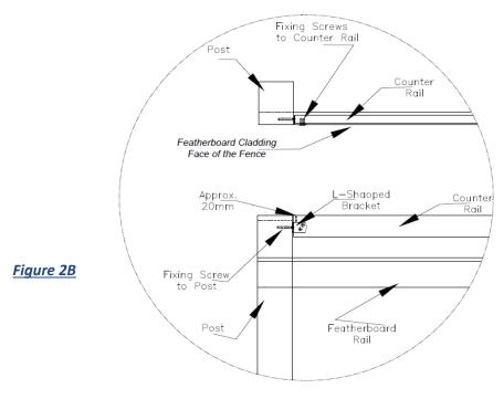
**11)** Next attach the counter rail to the inside face of the L shaped bracket, at both ends, using M4 x 25mm S/S countersunk screws as shown below (Ref: Figure 3)
