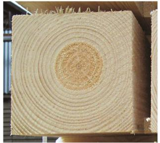
The cross section of an untreated timber post shown above shows the lighter sapwood surrounding the darker heartwood.
