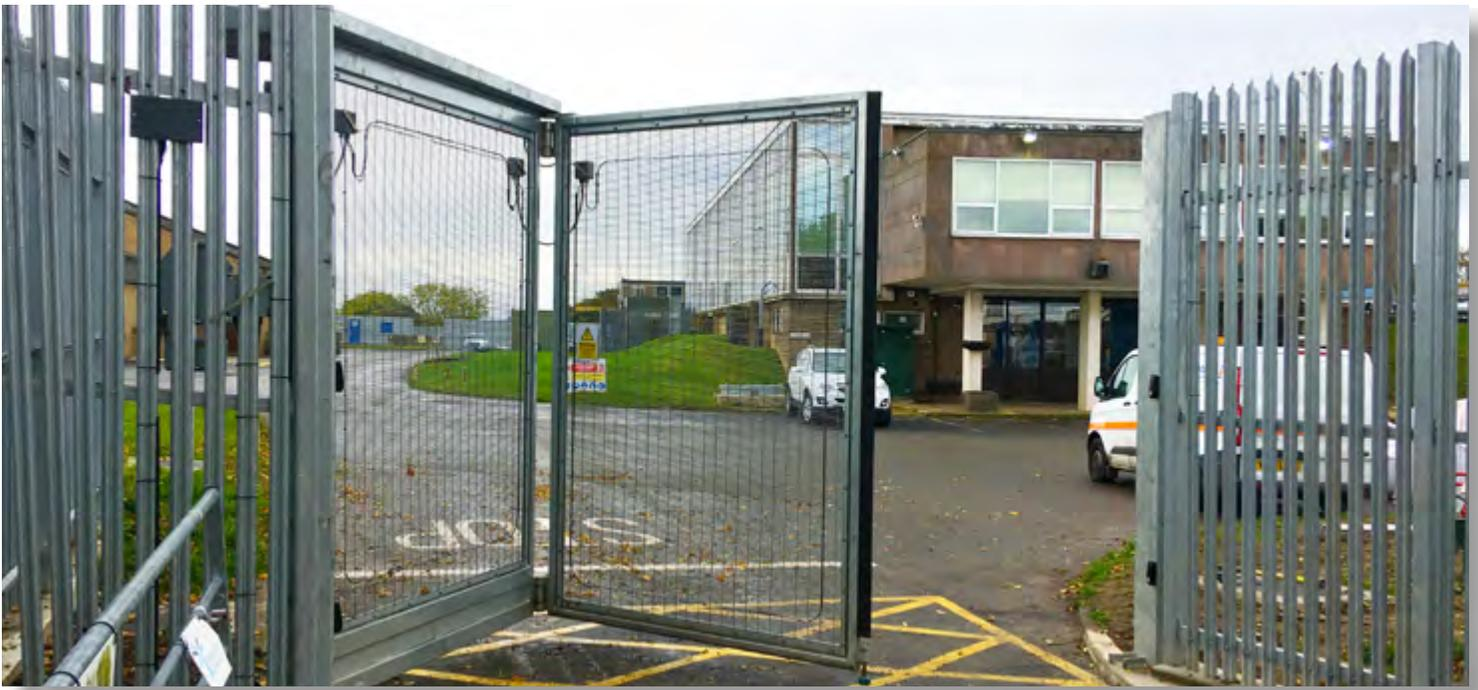
The trackless bi-folding speed gate comprises a unique drive mechanism to control the opening and closing of a bi-folding set of gates. The mechanism controls both leaves, producing a smooth and fast action. The design is ideal solution where the speed of opening and closing is essential for the security of the premises or where space may be a premium.
