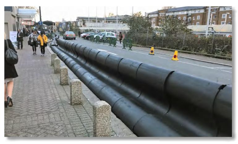
The Impakt Defender is an IWA14 rated vehicle security barrier (VSB) designed to protect people, buildings and infrastructure from hostile vehicle attack. Requiring no foundations, the surface mounted system can be rapidly deployed as a temporary or permanent security measure, as part of a robust hostile vehicle mitigation (HVM) strategy.
