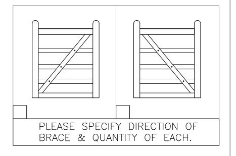
MANUFACTURE TOLERANCE  $\pm 5$ mm
