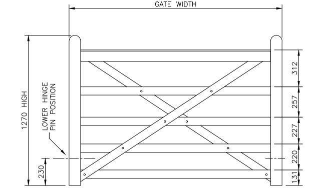
MANUFACTURE TOLERANCE  $\pm 5$ mm
