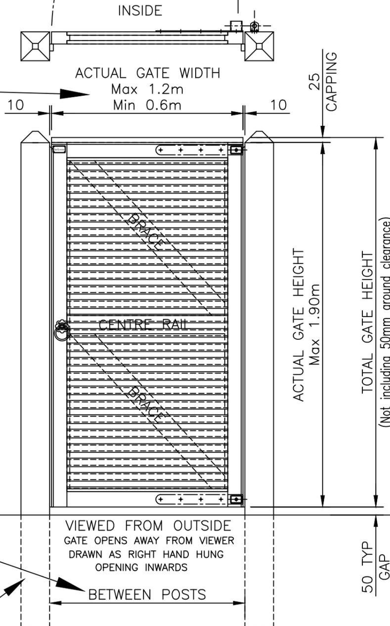
**NOTE:** Gate will be made with pales to be in line with Jacksons 'Venetian Hit & Miss' panels assuming the top of the gate capping will be inline with standard 20mm capping above 'Venetian Hit & Miss' panels. Kindly check for any other requirement.
