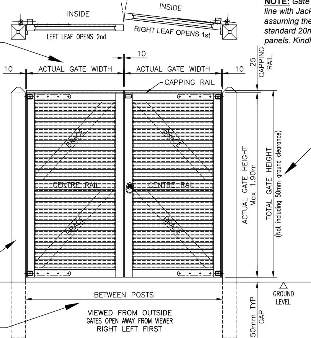
**NOTE:** Gate Leaf's will be made with pales to be in line with Jacksons 'Venetian Hit & Miss' panels assuming the top of the gate capping will be inline with standard 20mm capping above 'Venetian Hit & Miss' panels. Kindly check for any other requirement.
