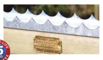
Sizes: Supplied in 1.80m lengths. The double row of spikes is 40mm wide and depth of spikes 25mm. Fixing: Security Comb comes drilled ready for fixing.
