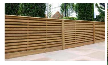
Constructed using 45mm x 16mm horizontal slats with a gap between the slats of approximately 30mm (which is larger than standard Venetian).
