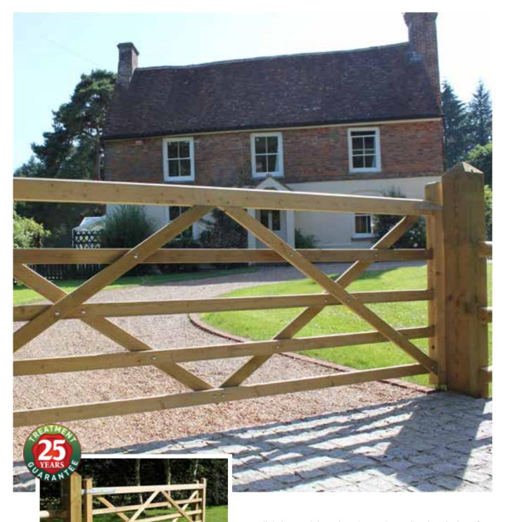
All timber used throughout is superior quality planed Jakcure® treated softwood guaranteed for 25 years. Top bars are chamfered and both hanging and slam stiles are drilled to allow gates to be hung on the left or right. Rail and brace crossings are bolted with stainless steel bolts. The gates are cross braced for extra strength and all joints are morticed and tenoned.
