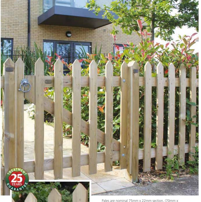
19mm planed finished size) planed with pointed or rounded tops with pale tops machined. When calculating materials required, you will need one post for every 2.28m plus one extra for the end of the run. There are 14 pales per bay. Each bay is backed by two 2ex 87 x 38mm nominal rails.
