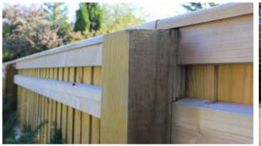
Posts are a nominal 125mm x 100mm in section for extra strength. The 1.20m fence posts feature two recesses, while the 1.50m and 1.80m versions have three recesses to accommodate the rails. Post tops are weathered in one direction. Supplied in a natural Jakcure® treated finish.
