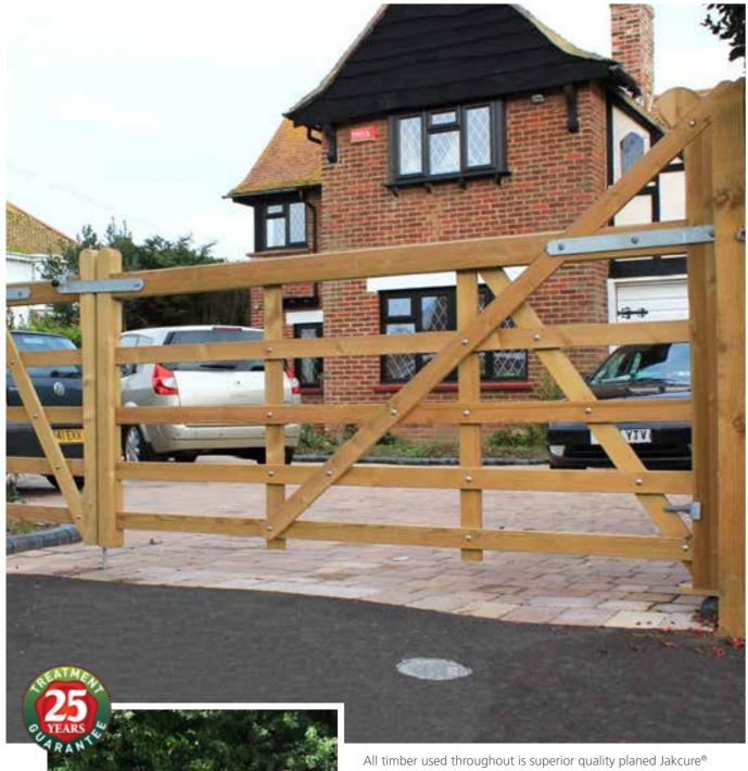
treated softwood guaranteed for 25 years. Rail and brace crossings are fixed with stainless steel bolts. The gates are cross braced for extra strength and all joints are morticed and tenoned.
