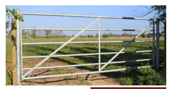
Specification: Gates are 1.15m high. Hanging stile of 50mm x 25mm box section. Slam stile of 50mm x 25mm box section. Top and bottom rails 41.5mm tube, with middle rails 32mm tube. Fittings include adjustable hinges and padlockable sliding latch. Also available with welded mesh cladding, (600mm high x 50mm x 50mm x 4mm) to the bottom part of the gate, please see below.
