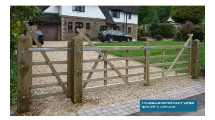
Gates are 1.20m high except for the hanging stile which is 1.50m. Hanging Stile 125mm x 75mm, Slam Stile 75 x 75mm, Top Rail is 100 x 75mm and under rail and cross braces 75mm x 25mm (all nominal). Supplied in natural Jakcure® finish. As standard, larger sizes are right hand hanging, smaller sizes are left hand hanging, see below for details.
