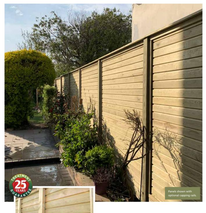
They feature a mortice and tenon jointed frame for extra strength while the infill is constructed using horizontal Tongue and Groove Effect boards. The centre of the panel is given additional support with one 70mm wide rail for heights up to 1.22m, and two rails for heights of 1.52m and above.
