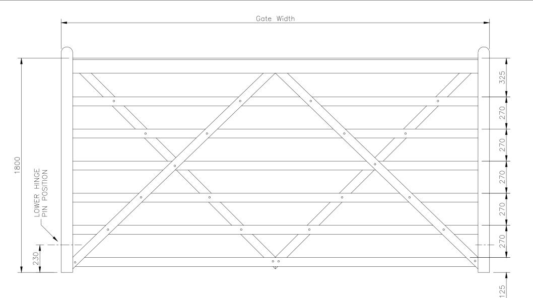
MANUFACTURE TOLERANCE  $\pm 5$ mm
