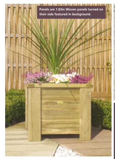
The 'L' formation corners are produced from 95mm x 22mm boards and the base consists of 95mm x 22mm slats with small drainage gaps with a planed finish. These sit approximately 80mm off the ground, on 38mm x 19mm battens.
