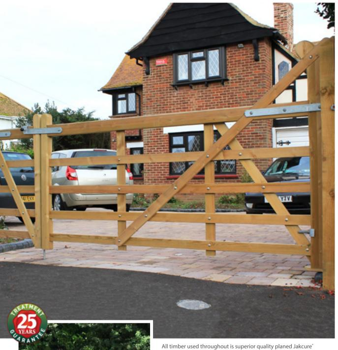
All timber used throughout is superior quality planed Jakcure\* treated softwood guaranteed for 25 years. Rail and brace crossings are fixed with stainless steel bolts. The gates are cross braced for extra strength and all joints are morticed and tenoned.
