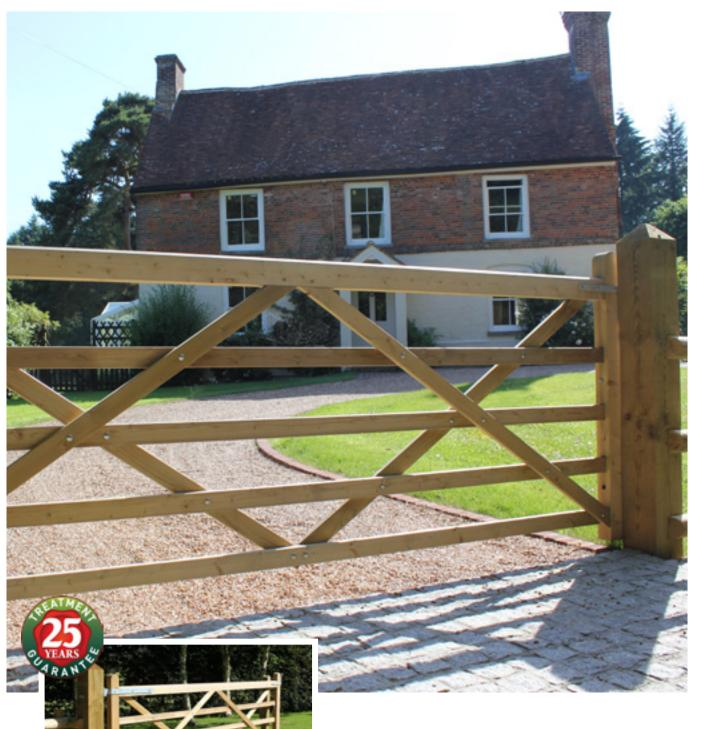
All timber used throughout is superior quality planed Jakcure® treated softwood guaranteed for 25 years. Top bars are chamfered and both hanging and slam stiles are drilled to allow gates to be hung on the left or right. Rail and brace crossings are bolted with stainless steel bolts. The gates are cross braced for extra strength and all joints are morticed and tenoned.
