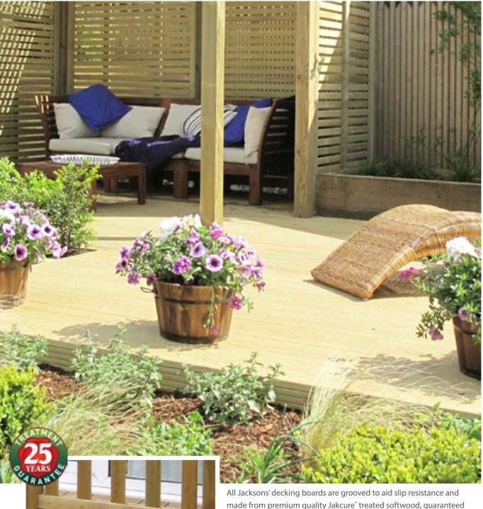
All Jacksons' decking boards are grooved to aid slip resistance and made from premium quality Jakcure treated softwood, guaranteed for 25 years. There are three board types available - Standard or Heavy Duty and slip resistant Heavy Duty.
