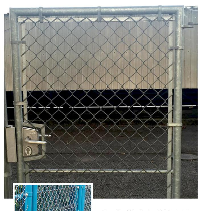
They are right or left hand hanging and clad with galvanised coated chain link, also available in a green finish. The framing is made from 42mm diameter galvanised tube. The gates come ready for hanging, complete with hinge pins, and bolts for attaching to the end strainer.
