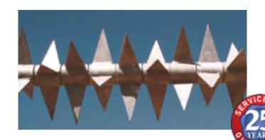
Sizes: Supplied in 6m lengths (shorter lengths available). Inner tube 41.5mm diameter. Blades 90mm long rotating on outer tube. 48.3mm diameter. Brackets at 3m centres when vertical and 2m when horizontal. Fixing: Brackets for fixing.
