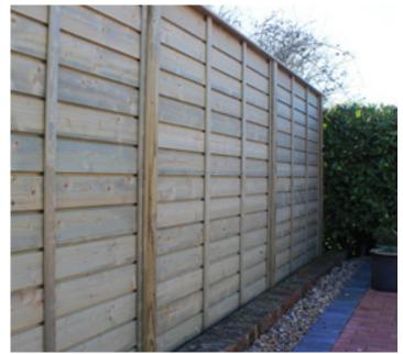
Shadowline panels are constructed using 'Z shaped' 144mm x 26mm horizontal boards which overlap. Each panel is manufactured using 4x 70mm x 24mm back rails.
